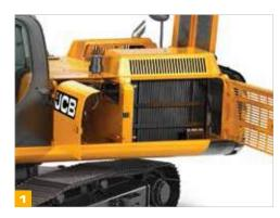
**1** JCB JS300 bonnet opens front-to-rear for easy and safe engine service access.
