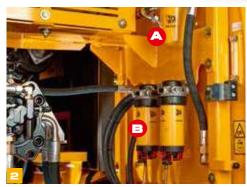
(A) Hydraulics oil filters (B) Fuel filters
